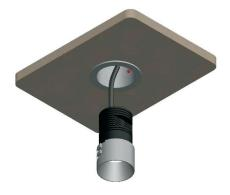
6 Insert the fixture though the installed base and turn it clockwise to lock it in desired position.
