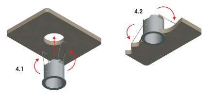
Insert the fixture though the installed base and turn it clockwise to lock it in desired position.
